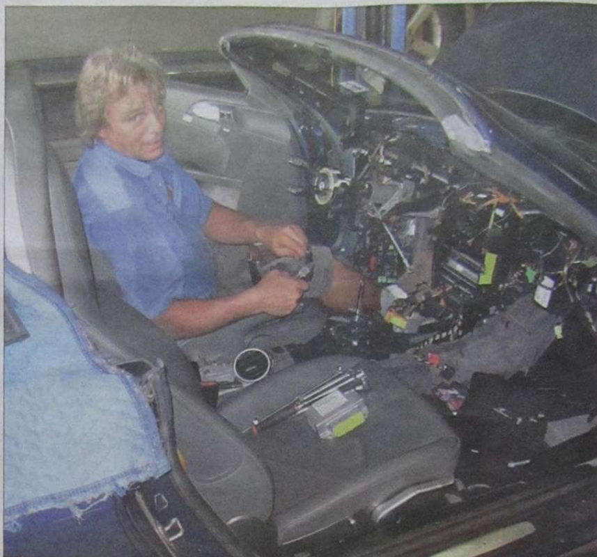
Tim Waits removing a Porsche instrument panel to replace an air conditioning evaporator, NOT an easy job!
